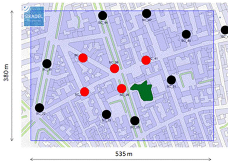
Figure 81. Small-cell network deployed in a dense urban environment (dots are small cell locations)
